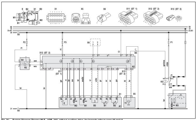
Fig. 21: System Diagram Thermo 90 S - ADR, 24V, without auxiliary drive, for legende refer to page 10 and 11
