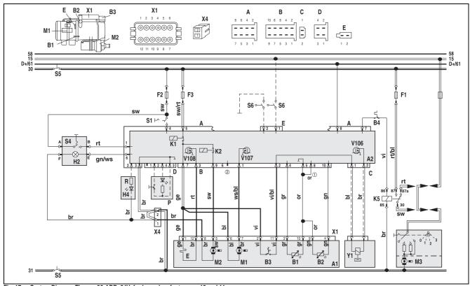
Fig. 17: System Diagram Thermo 90-ADR, 24V, for legende refer to page 10 and 11
