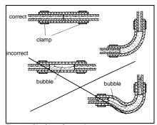
Fig. 9: Pipe/Hose Connection
