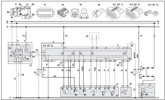
Fig. 19: System Diagram Thermo 90 S, 12 and 24V, with Digital Timer (standard) and circulating pump, for legende refer to page 10 and 11
