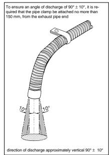
Fig. 13: Exhaust Pipe Discharge Opening
