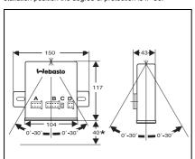
Fig. 14: Control Unit, Installation Position
