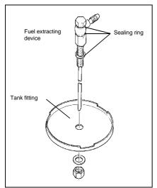
Fig. 5: Fuel Extraction From the Plastic Tank
