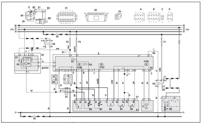
Fig. 16: System Diagram Thermo 90, 12 and 24V, with Digital Timer with 3 Time Settings, for legende refer to page 10 and 11
